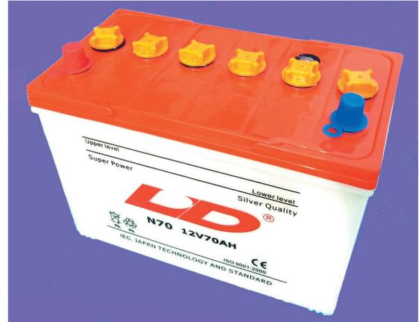
The typical automotive battery (often called a 12 Volt battery) actually consists of six (6) separate 2.1 Volt cells. These cells are connected in series and the individual cell voltages add up to create a total voltage. In the case of the automotive battery, six 2.1 Volt batteries in series make up a total voltage of 12.6 Volts.
