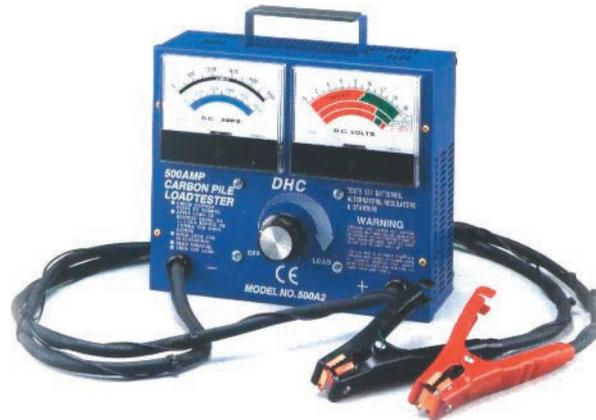
Based on what the voltage level drops to under load you can tell if the battery can be considered good or not. The main different between testing the voltage in the car under load and using a separate load tester is that the battery must be isolated from the vehicles electrical system prior to testing. This means that before using the load tester you should remove both battery cables from the battery terminals.
