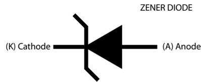
Also not typically used by installers, Zener diodes are used primarily in electronic circuits as a voltage regulation device. These devices, when wired in forward bias act as a regular junction diode. However, when wired in reverse bias, unlike the junction diode, current will pass through the diode once a certain amount of voltage is achieved. In other words, these diodes act as a voltage sensitive on/off switch.
