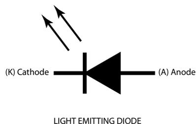
Light Emitting Diodes or LED's have many uses. Virtually all electronics equipment incorporates some LED's. Typically, they are used to provide the user with some form of information regarding the operation of the equipment.
