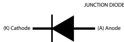
These diodes are used primarily for circuit isolation or rectification. They come in several shapes and sizes depending on the application.
