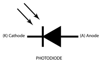
Although not used by installers, photo diodes are part of the diode family and should be briefly discussed. These types of diodes conduct current when energized by light energy. Think of the light as an on/off switch for the diode. Typically used to turn on a night light at night.
