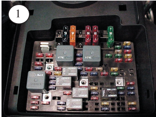
Here are some examples of newer vehicle fuse panels using Mini (ATM) and MAXI fuse applications. Photo 1 shows the under hood fuse and relay panel in a 2001 Chevrolet Corvette. Photo 2 shows the interior fuse panel (located behind the drivers side dash) in a 2000 model Toyota Corolla
