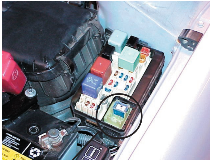
An example of a JCASE (FMX) fuse in a under hood application on a Toyota vehicle
