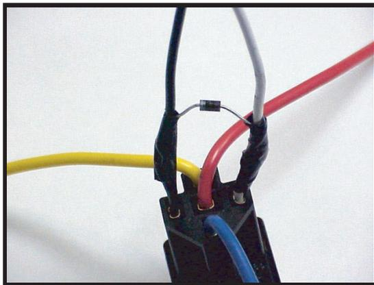
Tape connection between diode and wires.
