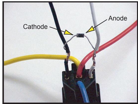
Attach diode to wires. Cathode - Terminal 86 +
