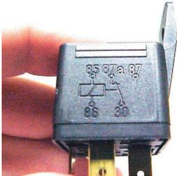
The “schematic” for how the relay functions is located on the side or top of every relay. This Bosch relay shows terminals 30 and 87a connected while it's in the rest or off position. When the relay switches on, you can see that 30 and 87 become connected, while 87a becomes disconnected. 30 is connected to something all of the time.
