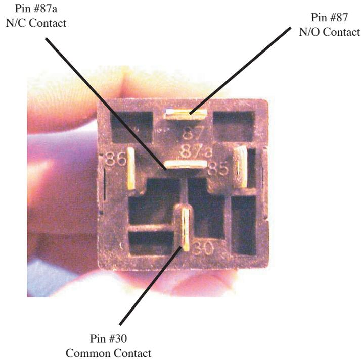
A look at the back of a Bosch relay and terminals 30, 87a, and 87. Actual connections are soldered onto these terminals or a custom wired harness is plugged into the back of the relay.
