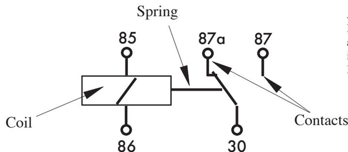
A look at the schematic of a Bosch SPDT relay as pictured above. This schematic is illustrated on the side of each Bosch relay
