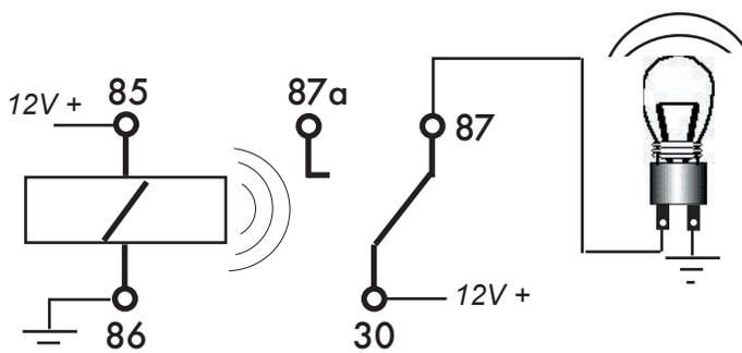
In this diagram the coil of the relay has been energized and has caused contact between terminals 30 and 87. As a result the bulb lights up and will remain lit until the coil side of the relay is de-energized.
