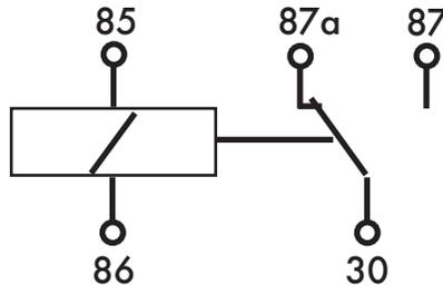
In this diagram terminal 30 is connected to terminal 87a, this is the normal or (off) state of the relay and will remain this way until the coil is energized.
