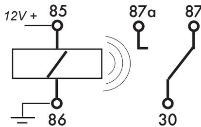
In this diagram the coil side of the relay has been energized. As a result, a magnetic field has effected the spring and caused the common terminal (30) to disconnect from terminal 87a and instead make contact with terminal 87.
