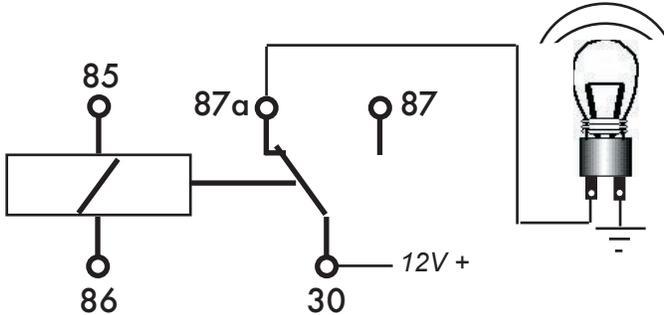
In this diagram the light bulb is lit and will remain lit until the coil side of the relay has been energized. This is a common turn off circuit. If controlled by the alarm system the bulb would shut off when activated by a signal from the alarm system.
