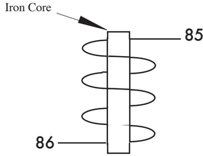
A coil is a device that when connected to a power source and ground will produce a magnetic field.
