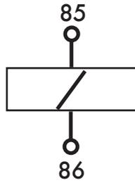
The coil side of a typical automotive SPDT relay as seen on the schematic located on side of the relay
