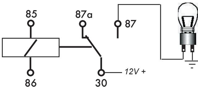
In this diagram the light bulb positive lead has been connected in series with terminals 30 and 87. In its current off state the relay does not allow the 12V+ signal to travel to the light bulb. The bulb will not light regardless of the fact that is connected permanently to ground.
